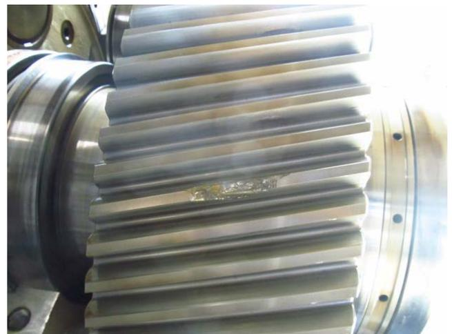
**Fig. 13** Cracked big gear on sun shaft in IS
