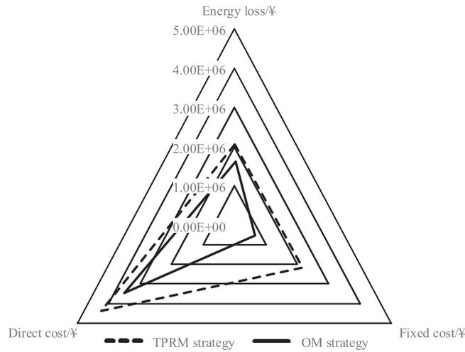
**FIGURE 7** Components of the total maintenance cost under the two strategies
