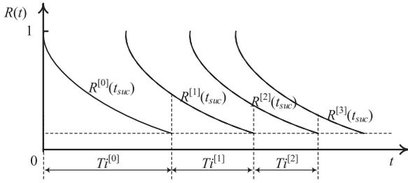
**FIGURE 3** Reliability variation of the subassembly under the imperfect maintenance
