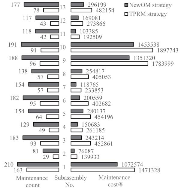
**FIGURE 5** Expected maintenance count and cost of each subassembly under the two strategies
