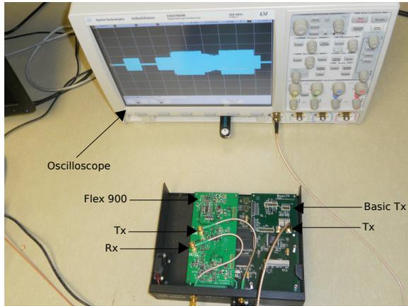
Figure 9: Photograph of measurement setup.
