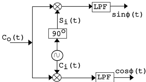
Figure 6: Oscillator offsets with reference signal.
