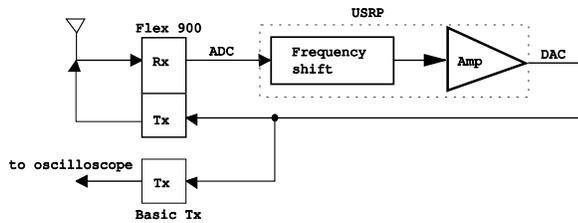
Figure 8: Measurement setup for beamforming experiment.
