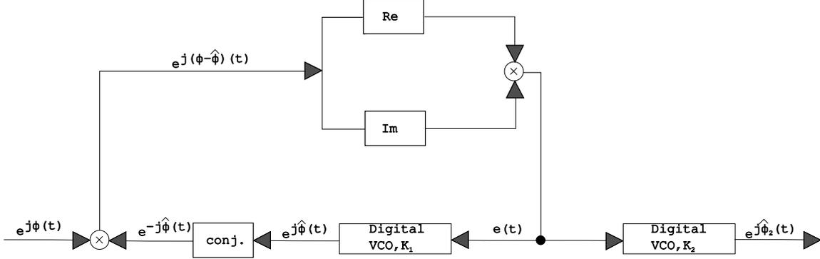
Figure 7: Modified baseband Costas loop for frequency-locking.
