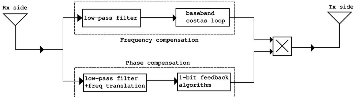
Figure 4: Signal processing at the Slave nodes.
