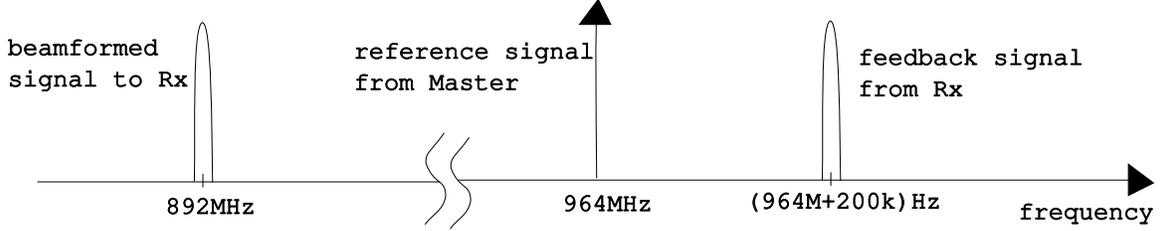
Figure 5: Frequency multiplexing scheme for beamforming experiment.
