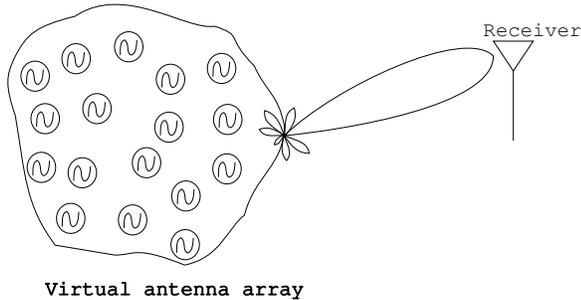
**Figure 1: Energy efficient transmission using distributed beamforming.**
