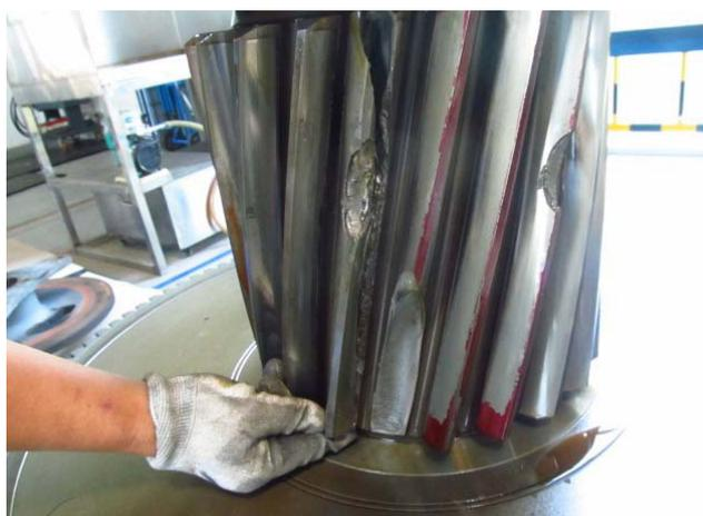
**Fig. 11** Broken gear on intermediate shaft in IS
