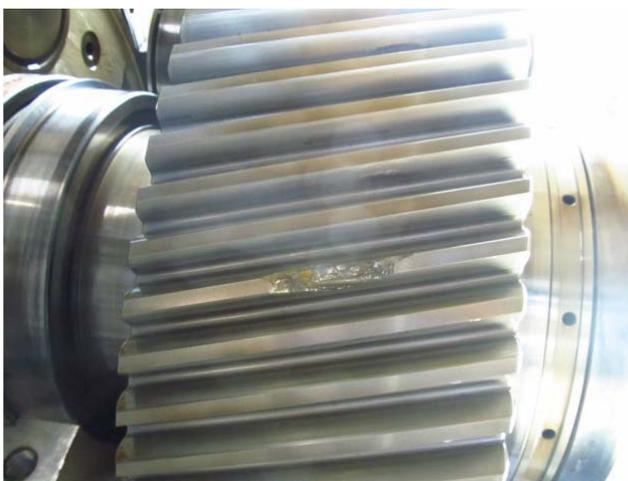
**Fig. 13** Cracked big gear on sun shaft in IS
