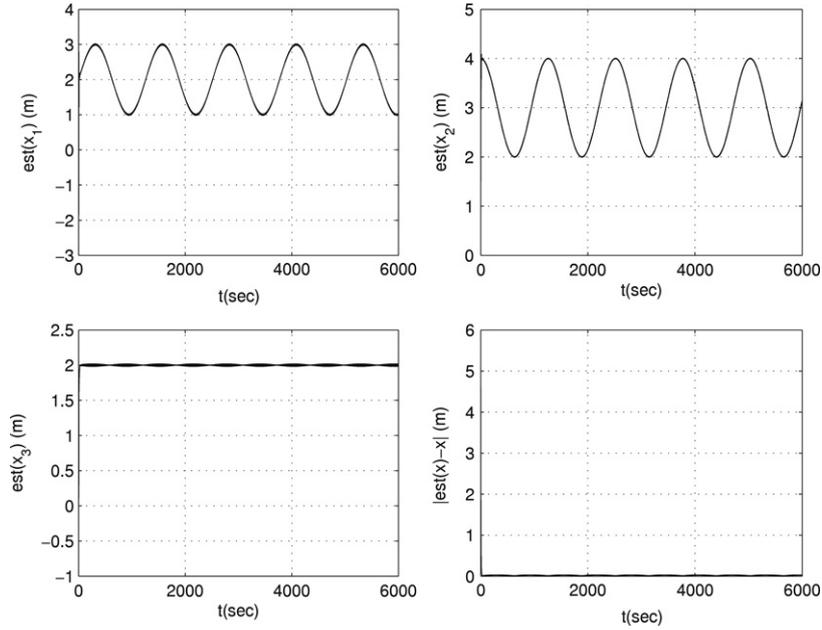
**Fig. 2.** Location estimation for  $x(t) = [2 + \sin 0.005t, 3 + \cos 0.005t, 2]^T$  (m),  $y(t) = [2 + 2 \sin t, 2 \cos 2t, 2 \sin 0.5t]^T$  (m),  $\alpha = 1$ . The dashed curves correspond to the actual coordinates of the source and the solid curves show the estimate trajectories. Time scale 0–6000 s.
