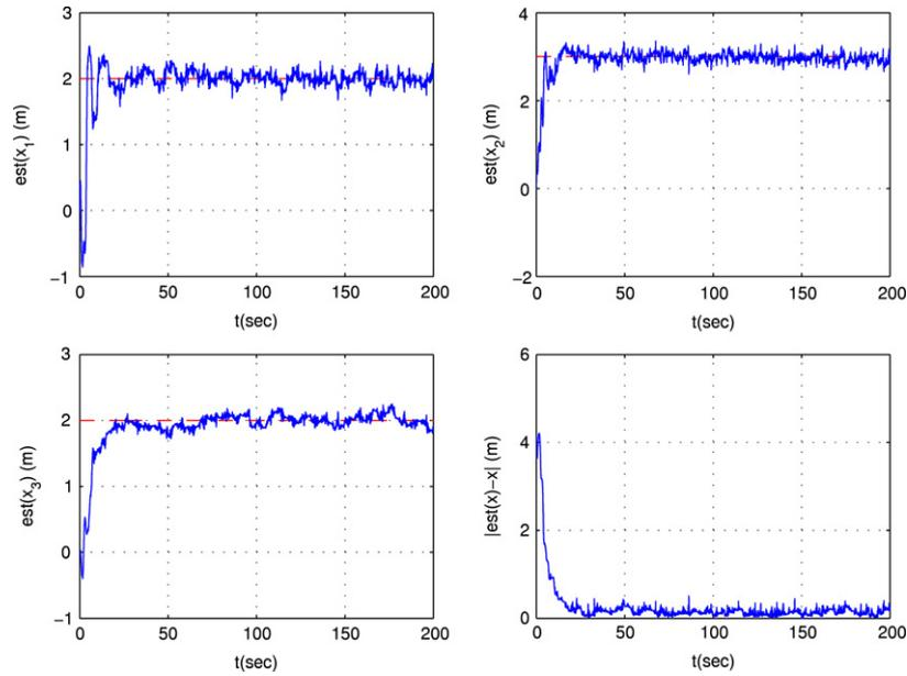
**Fig. 5.** Location estimation for  $x = [2, 3, 2]^T$  (m),  $y(t) = [2 + 2 \sin t, 2 \cos 2t, 2 \sin 0.5t]^T$  (m),  $\alpha = 1$ . Noise in distance measurement with power  $.001$  ( $\text{m}^2$ ). The dashed lines correspond to the actual coordinates of the source, and the solid curves show the estimate trajectories.
