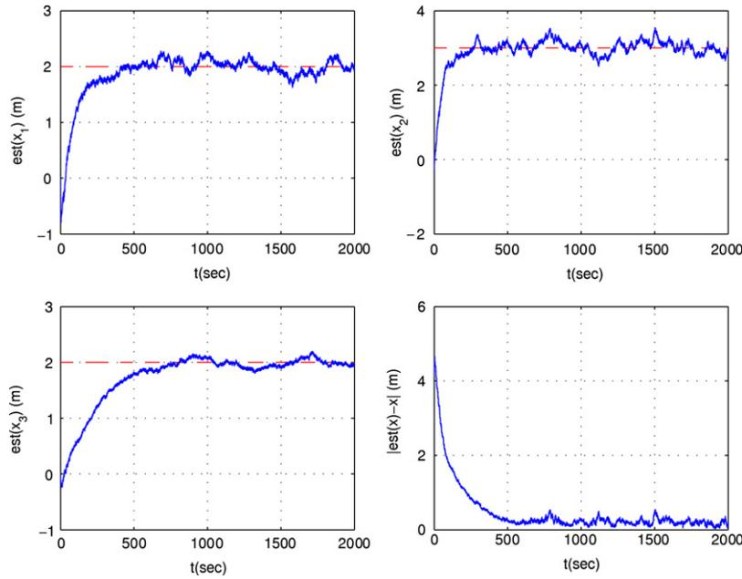
**Fig. 7.** Location estimation for  $x = [2, 3, 2]^T$  (m),  $y(t) = [2 + 2 \sin t, 2 \cos 2t, 2 \sin 0.5t]^T$  (m),  $\alpha = 1$ . Noise in distance measurement with power  $0.1$  ( $\text{m}^2$ ) and adaptation gain  $0.01$ . The dashed lines correspond to the actual coordinates of the source, and the solid curves show the estimate trajectories.
