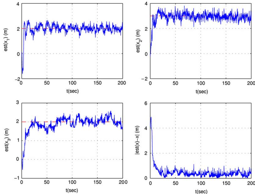
**Fig. 6.** Location estimation for  $x = [2, 3, 2]^T$  (m),  $y(t) = [2 + 2 \sin t, 2 \cos 2t, 2 \sin 0.5t]^T$  (m),  $\alpha = 1$ . Noise in distance measurement with power  $.005$  ( $\text{m}^2$ ). The dashed lines correspond to the actual coordinates of the source, and the solid curves show the estimate trajectories.
