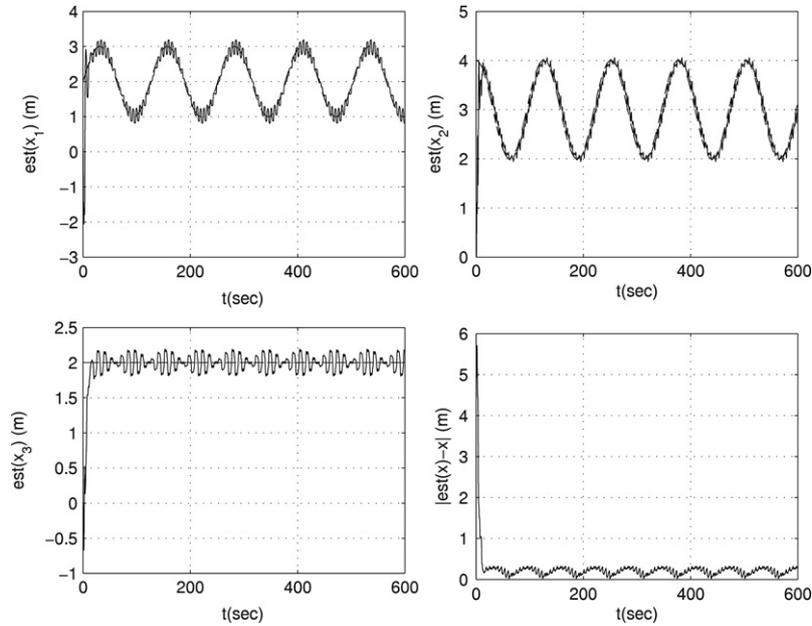
**Fig. 4.** Location estimation for  $x(t) = [2 + \sin 0.05t, 3 + \cos 0.05t, 2]^T$  (m),  $y(t) = [2 + 2 \sin t, 2 \cos 2t, 2 \sin 0.5t]^T$  (m),  $\alpha = 1$ . The dashed curves correspond to the actual coordinates of the source, and the solid curves show the estimate trajectories. Time scale 0–600 s.
