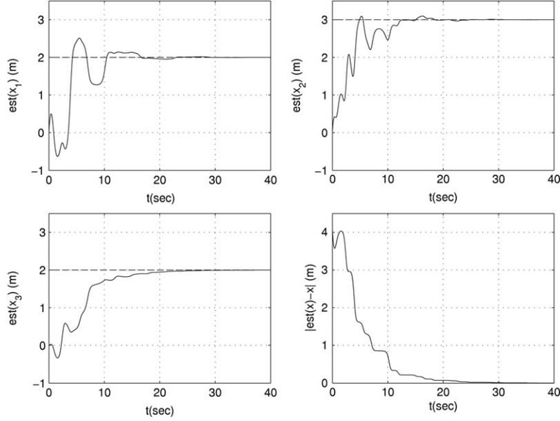
**Fig. 1.** Location estimation for  $x = [2, 3, 2]^T$  (m),  $y(t) = [2 + 2 \sin t, 2 \cos 2t, 2 \sin 0.5t]^T$  (m),  $\alpha = 1$ . The dashed lines correspond to the actual coordinates of the source and the solid curves show the estimate trajectories.
