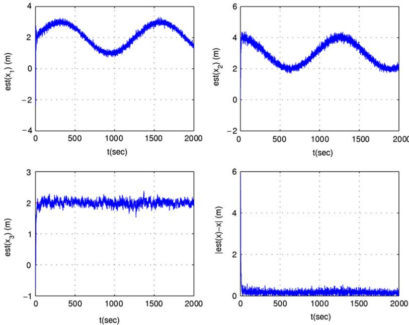
**Fig. 8.** Location estimation for  $x(t) = [2 + \sin 0.005t, 3 + \cos 0.005t, 2]^T$  (m),  $y(t) = [2 + 2 \sin t, 2 \cos 2t, 2 \sin 0.5t]^T$  (m),  $\alpha = 1$ . Noise in distance measurement with power  $0.001$  ( $\text{m}^2$ ). The dashed lines correspond to the actual coordinates of the source, and the solid curves show the estimate trajectories.
