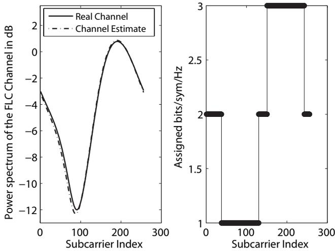
Fig. 5. Multipath channel frequency response and bit loading result using [4].
