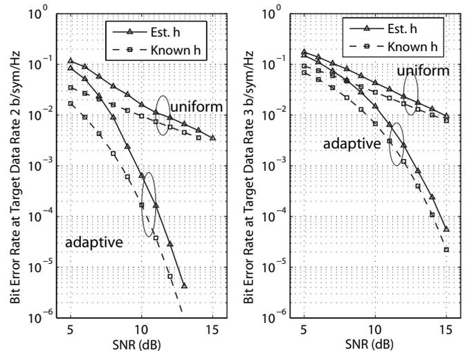
Fig. 8. Bit error rate comparison of a bit loaded and uniformly modulated static OFDM system with different target data rates.
