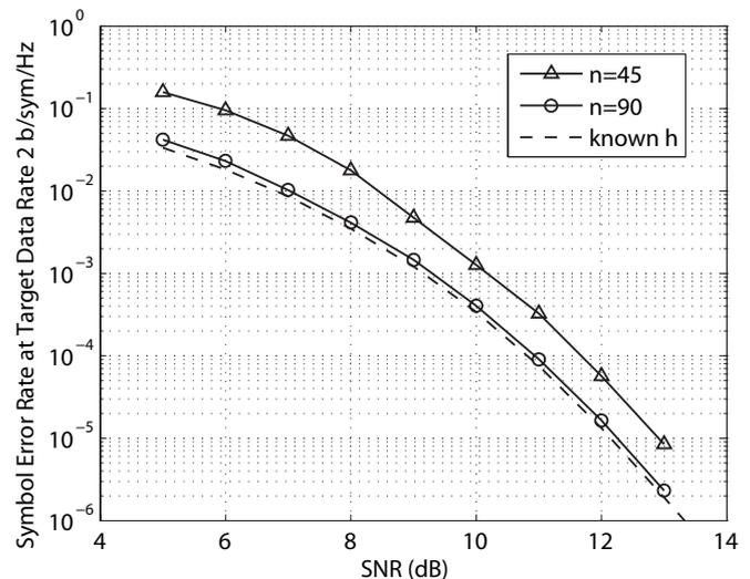
Fig. 9. Symbol error rate comparison of a bit loaded static OFDM system using different feedback data length.
