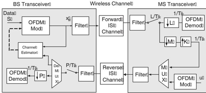
Fig. 2. An OFDM system with decimated feedback.
