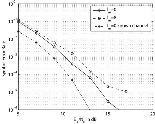
Fig. 10. Symbol error rate performance of an OFDM system with a slowly time-varying channel.
