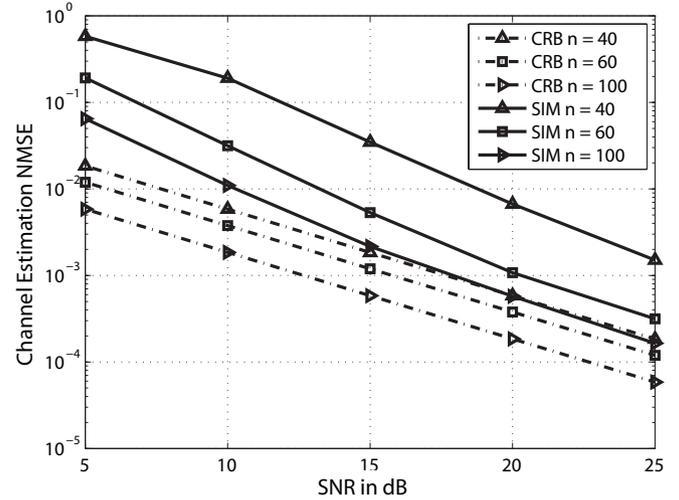
Fig. 6. Forward link channel estimation Cramer Rao lower bound v.s. simulated NMSE.
