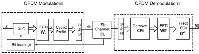
Fig. 1. A DFT-based OFDM system with cyclic-prefix.
