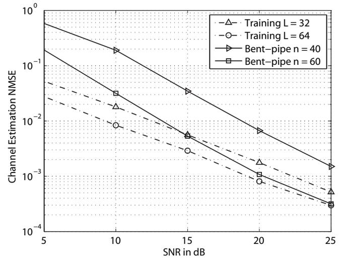
Fig. 7. Comparison of the training based method and the bent-pipe feedback method.
